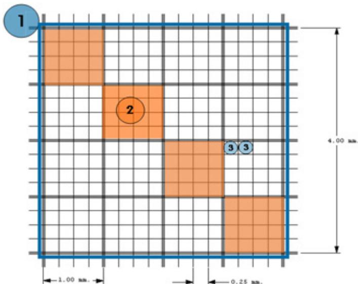
**Fig. 1:** Layout of a Fuchs Rosenthal Counting chamber
